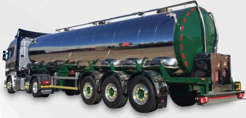
From remounting a rigid tanker on to a new chassis cab, refurbishing or replacing operational equipment and repainting to replacing a full set of trailer running gear anything is achievable. We can modify your existing vehicle to suit contract requirements if they change with pump upgrades for a change in the product to be carried or just performance, we also offer ADR tank testing and re certification for a change of use, call us for more information and to discuss your needs and requirements.
