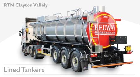
These tankers are mostly designed for the chlor-alkali industry and can be lined in natural and synthetic rubbers and also glass and fluoropolymer lined.
