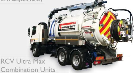
The RCV ultra max combination units are based on a successful design which has been tried and tested for 20 plus years but has evolved to suit our customers ever growing demand for more performance but still maintaining a compact, easy to operate and reliable design. The RCV combination units start from 7.5 tonne to 32 tonne and are available from 300 cfm to 7,000 cfm vacuum capability and jetting from 9 gpm to 150 gpm depending on the size of the vehicle.
