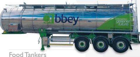
Working to very exacting standards to ensure the highest standard of internal finish, these tank types are designed to transport a full range of edible products, including oils, chocolate, beer, whisky, milk, etc. Full C I P is fitted and air filtration is a standard feature. Central sequential locking is an option fitted to offer maximum security of product. Temperature control is fitted were necessary to ensure the complete integrity of the product.
